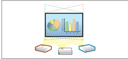
These projectors provide vertical (automatic/manual) and horizontal (manual) keystone correction. Thanks to these functions, it is not necessary to put the projector in the center of the desk. You can place the projector anywhere you want.
