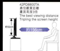
▲ 屏幕高度約52cm x 3 = 最佳視聽距離 The best viewing distance = 3 x screen height (52cm)
